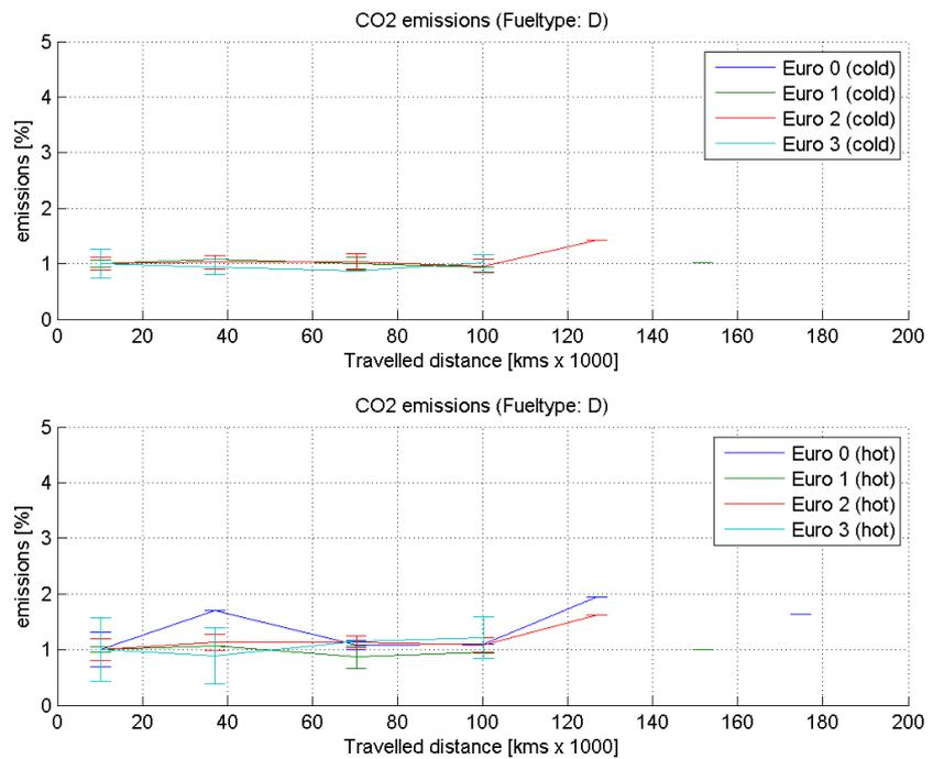
Figure 15 CO<sub>2</sub> test results of diesel vehicles as a function of the vehicle distance travelled (1=100%).
