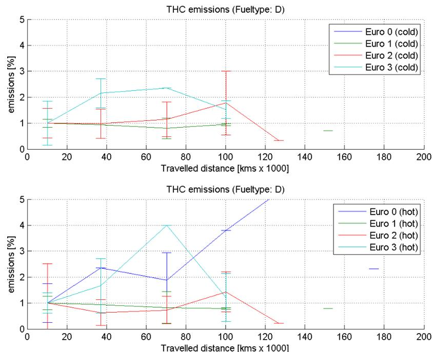
Figure 13 THC test results of diesel vehicles as a function of the vehicle distance travelled; respectively cold and hot NEDC cycle (1=100%).
