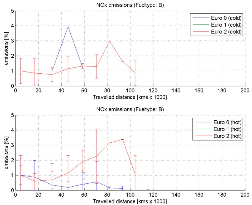
Figure 12 NO<sub>x</sub> test results of petrol vehicles as a function of the vehicle distance travelled (1=100%).
