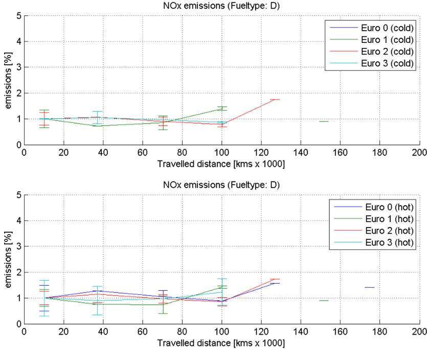
Figure 16 NO<sub>x</sub> test results of diesel vehicles as a function of the vehicle distance travelled (1=100%).
