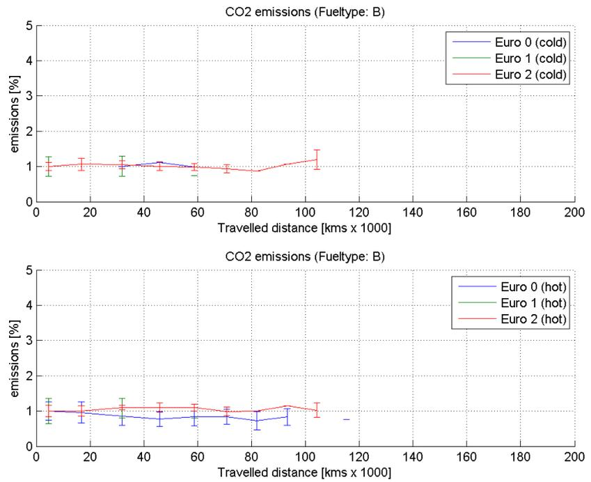
Figure 11 CO<sub>2</sub> test results of petrol vehicles as a function of the vehicle distance travelled (1=100%).
