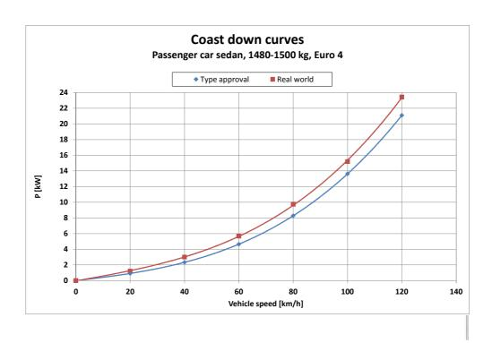
Figure 15: Type Approval and realistic road load curve of vehicle 1 (my 2008)
