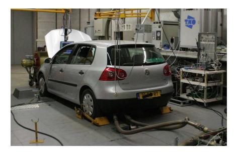
Figure 5: Chassis dynamometer or roller bench
