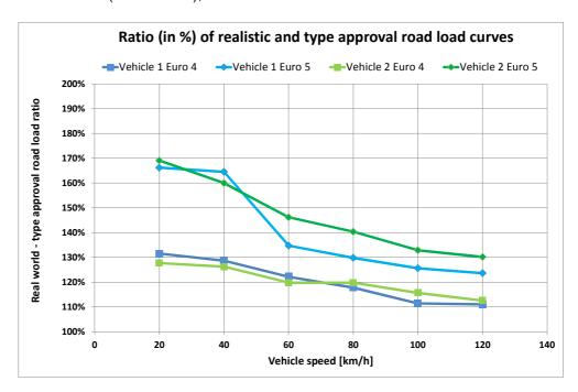
Figure 7: Road Load Ratios of 2 vehicles, both as Euro 4 and 5 configuration (TA = 100%)
