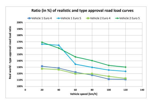
Figure 2: Road Load Ratios of 2 vehicles, both tested as Euro 4 and 5 configuration (TA = 100%)
