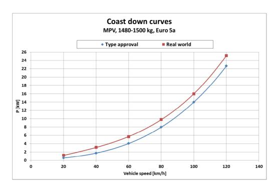
Figure 21: Type approval and realistic road load curve of vehicle 5
