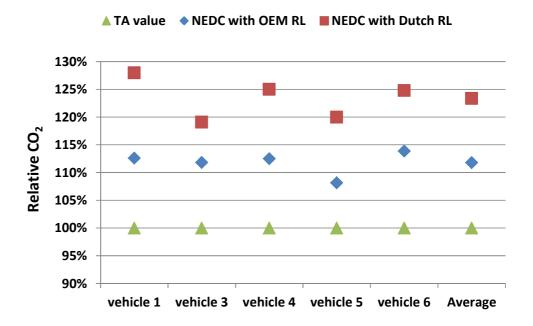
Figure 3: Relative CO<sub>2</sub> emissions of Euro 5 and 6 vehicles in a NEDC test with different road load settings
