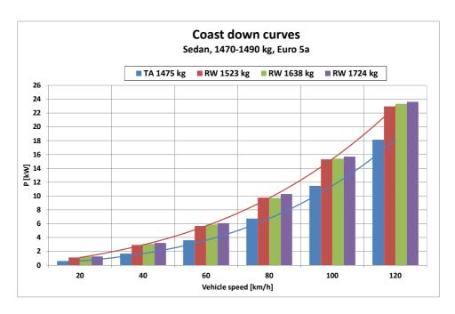
Figure 9: Type approval and realistic road load curves with different vehicle masses of vehicle 6
