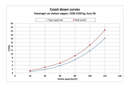
Figure 16: Type Approval and realistic road load curve of vehicle 1 (my2012)
