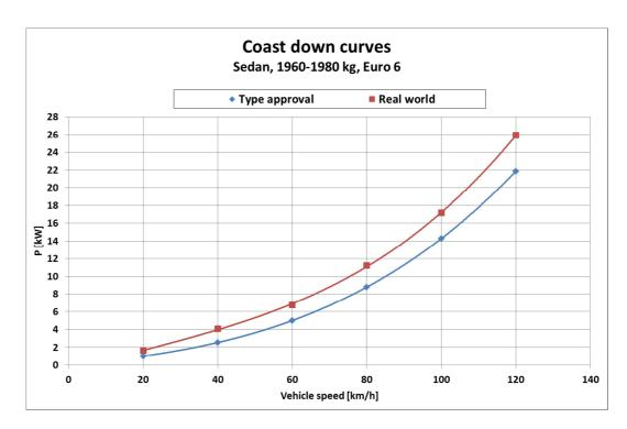
Figure 20: Type Approval and realistic road load curve of vehicle 4
