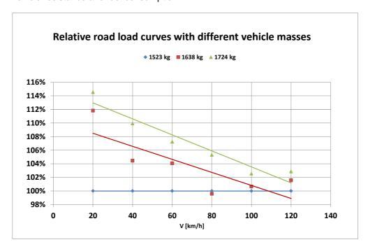
Figure 10: Relative differences road load curves (vehicle mass 1523 kg = 100%)
