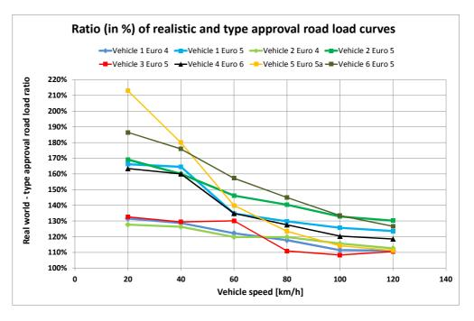
Figure 6: Ratio of TA+RW road load test results of all tested vehicles
