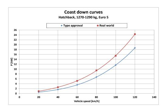
Figure 18: Type Approval and realistic road load curve of vehicle 2 (my2012)
