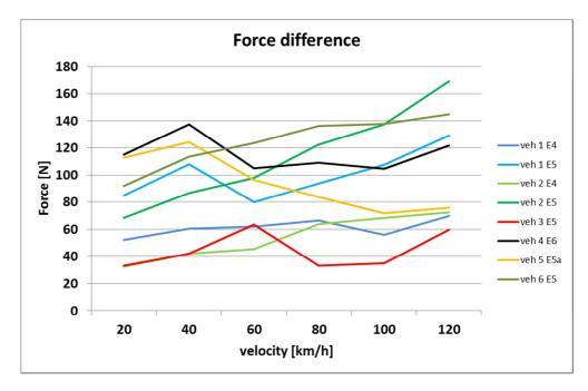
Figure 14: The force difference between the Type Approval value and the tests, the Euro-4 vehicles (1 and 2) have a force difference between 30 and 70 N, while most modern vehicles have values typically twice this value, with the exception of vehicle 3.
