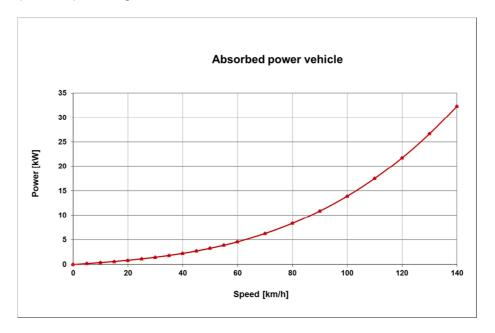
Figure 11: Example vehicle absorbed power curve
