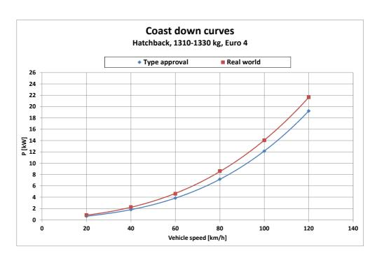
Figure 17: Type Approval and realistic road load curves of vehicle 2 (my2009)
