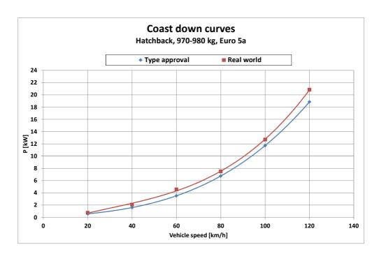
Figure 19: Type Approval and realistic road load curve of vehicle 3
