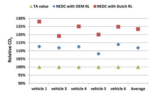
Figure 8: NEDC CO<sub>2</sub> emissions of Euro 5 and 6 vehicles with different road load settings
