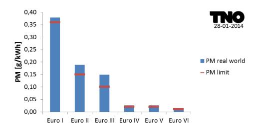
Figure 8: PM real world emissions and type approval limit values of heavy duty vehicles.
