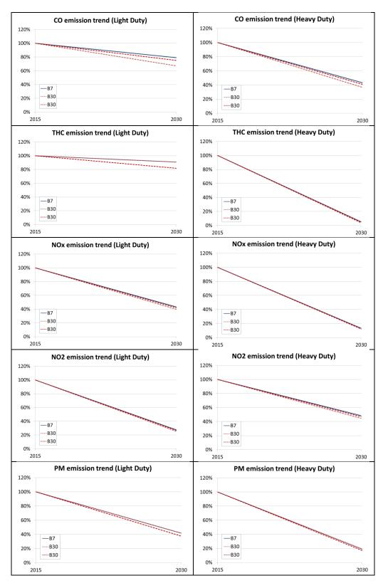
Figure 1: Predicted emissions trends 2015-2030 – Light Duty and Heavy Duty vehicles and the effects of increased biodiesel blends.
