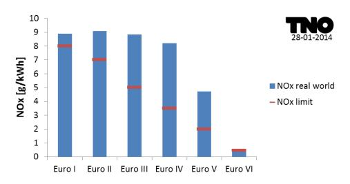
Figure 7: NOx real world emissions and type approval limit values of heavy duty vehicles.
