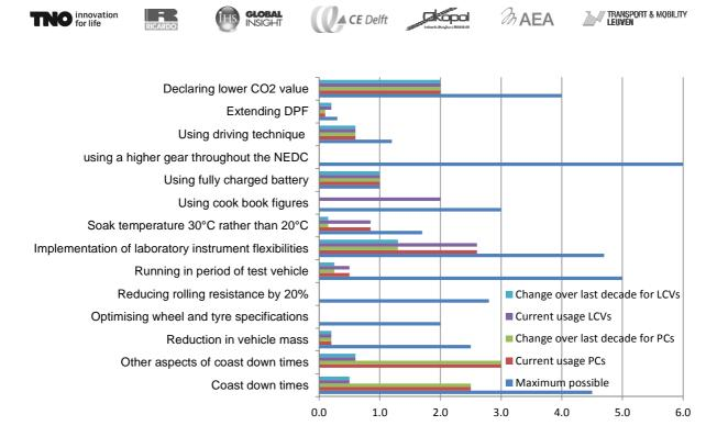
Figure 19 Bar graph of the current extent to which flexibilities reduce CO<sub>2</sub> emissions for light duty vehicles
