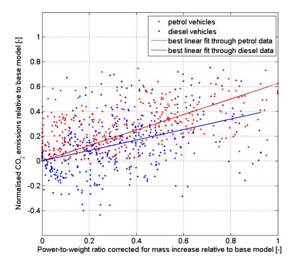
Figure 26 Relation between the power-to-weight ratio and the CO<sub>2</sub> emissions for passenger cars on petrol and diesel
