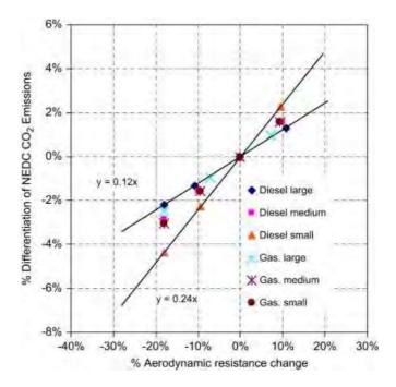
Figure 12 Effect of aerodynamic resistance on NEDC CO<sub>2</sub> emissions for a range of vehicle categories
