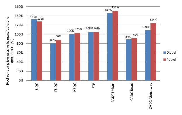
Figure 9 Variation of fuel consumption between different test cycles (UDC = Urban Drive Cycle - EUDC = Extra Urban Driving Cycle - NEDC = New European Driving Cycle - FTP = Federal Test Procedure - CADC = Common Artemis Driving Cycle
