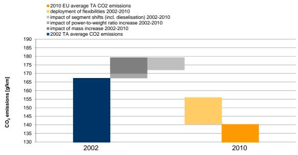
Figure 23 Result of the bottom-up analysis with respect to the possible contribution of increased utilisation of test flexibilities to the observed reduction of CO<sub>2</sub> emissions from passenger cars between 2002 and 2010
