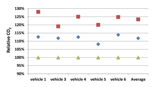
▲ TA value ◆ NEDC with OEM RL ■ NEDC with Dutch RL
