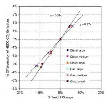
Figure 11 Effect of vehicle weight on NEDC CO<sub>2</sub> emissions for a range of vehicle categories. Trend-lines correspond to the vehicles affected the most and the least by weight change.
