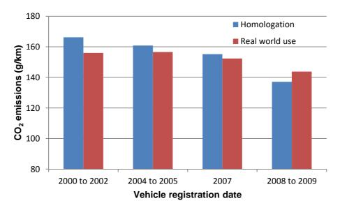
Figure 20 Average CO2 emissions from diesel vehicles at homologation and from real world use against vehicle registration year<sup>16</sup>
