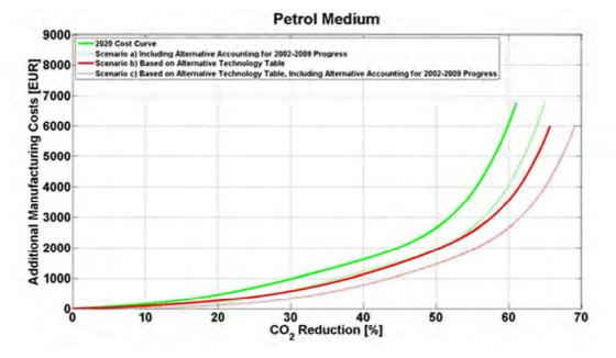
Figure 4 Example of the main cost curves and scenario variants used in the assessment of the impacts of the 2020 target for passenger cars in [TNO 2011].
