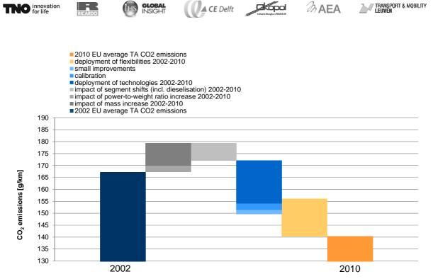
Figure 24 Graphical summary of the top-down and bottom-up analysis of the contributions of technology deployment resp. test cycle flexibilities to the reduction of passenger car CO<sub>2</sub> emissions observed between 2002-2010
